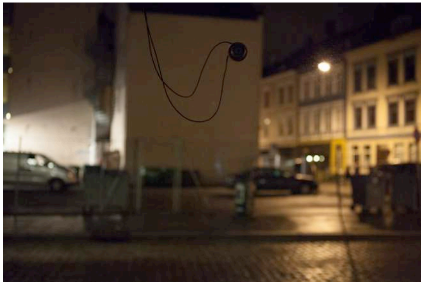
Figure 57, Detail: Transducer turning the window into a loudspeaker, seen from the inside.
