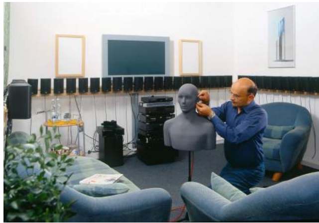
Figure 3.16: Wave field synthesis test setup at the Fraunhofer Institute for Digital Media Technology IDMT in Ilmenau for the Carrouso research project 2001-2003 ( http://www.emt.iis.fraunhofer.de/projects/carrouso ).
